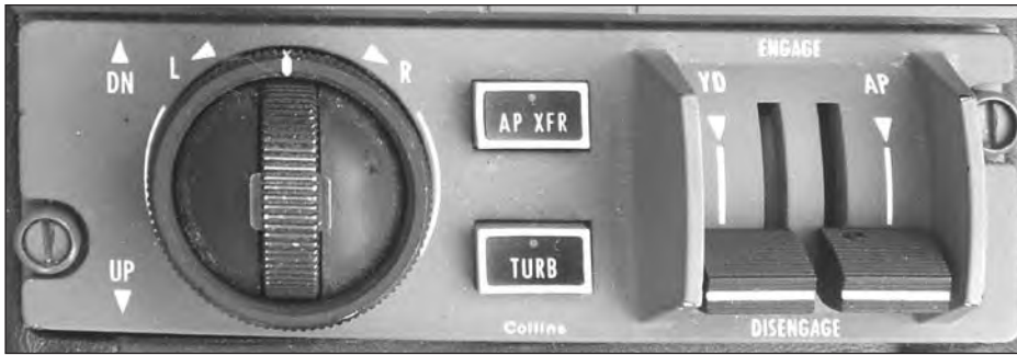
Autopilot control head on a Cessna Citation II; the yaw damper and autopilot engage switches are side-by-side.
