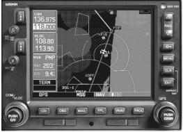
A combination of an Aspen EFD1000 (left) and a pair of Garmin GNS530W navigators (one shown above) creates the basis of nearly a full glass cockpit upgrade. However, it's essential to know how the units integrate with each other and the rest of the avionics in the airplane before you fly IFR.
